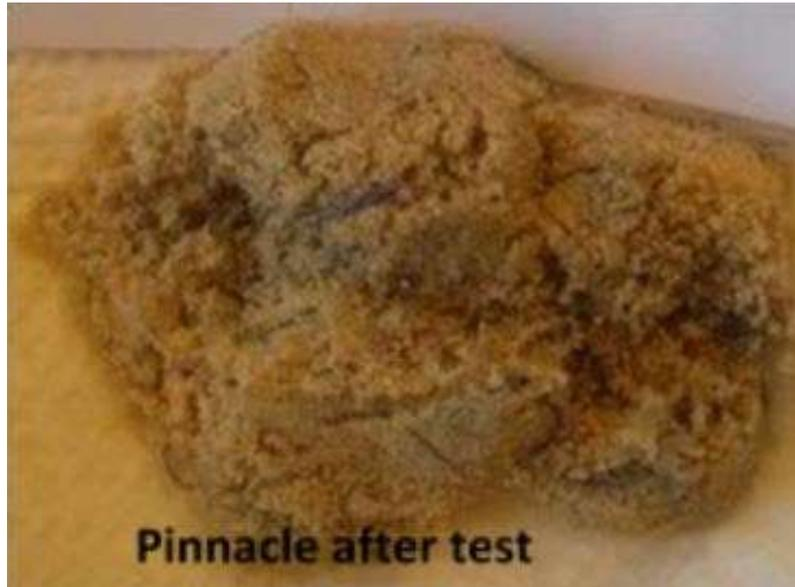
Attwood's Pinnacle polymer coated surface after the same test shows no deterioration.
