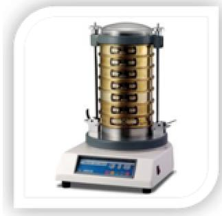
The largest grains are retained on the sieve with the largest holes whilst the smaller grains can fall through these to be retained on the sieves below with smaller holes. This grain size distribution is very important in partly defining the final properties of the surface. Another is the amount of additive such as fibre or fabric/felt incorporated into the sand, and this can be measured by separating the sand from the additive and weighing the two fractions.
