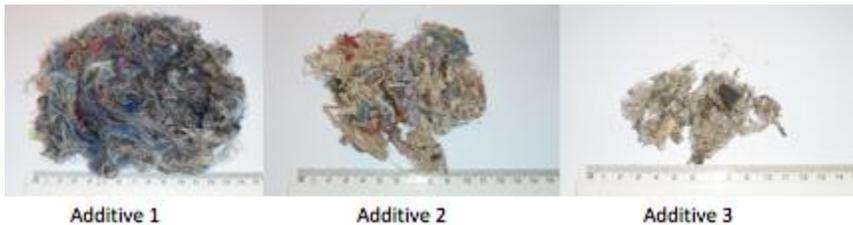
Take a look at a range of commercially available additives in the pictures. Firstly note how separated the fibres are. In the case of Additives 2 & 3, the fibre is in the form of carpet yarn where the individual fibres are designed to stay within the yarn tufts by twisting and setting - this is what you want from a carpet, but not what you want for footing!
